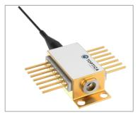
As a tapered amplifier, the *miniTA* has a fiber-coupled input and collimated output beam and is available in an optimized butterfly package with 14 thicker pins starting in February. This hermetically sealed housing is particularly advantageous in industrial applications, as the thicker pins guarantee an ideal supply of power. Furthermore,
